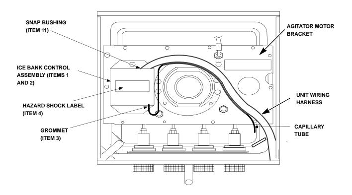
FIGURE 3. UNIT TOP VIEW
